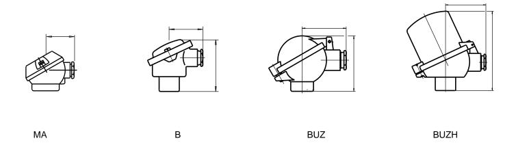
Form MA, aluminium die-casting, M6\*1.5; IP65, ambient temperature -40 to +100° C
